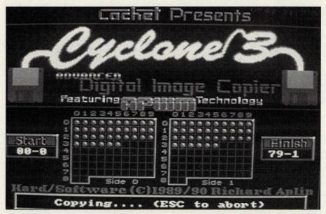
The Cyclone III disk backup requires a hardware dongle and a second disk drive. It will duplicate a disk from one drive to the next.
